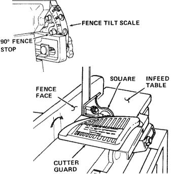
b. Loosen 90° stop screw with small screwdriver and turn knurled sleeve which will cause fence to tilt. Turn sleeve in either direction until fence is square with infeed table.
